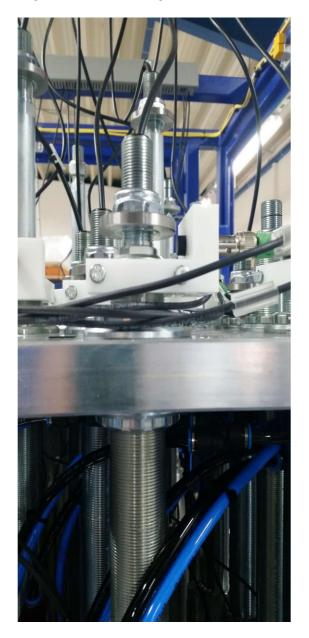
Welding actuators with horns
